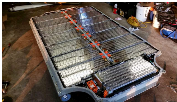
Obr. 1 Batéria elektromobilu Tesla Model S - 85 kWh [1]
