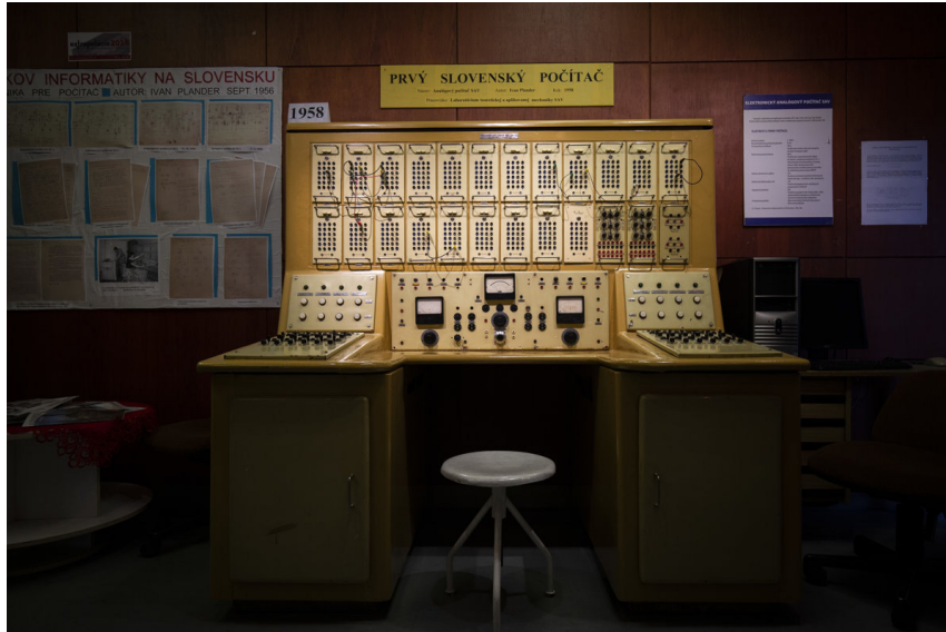
Fig. 1 First slovak analog computer. [2]
