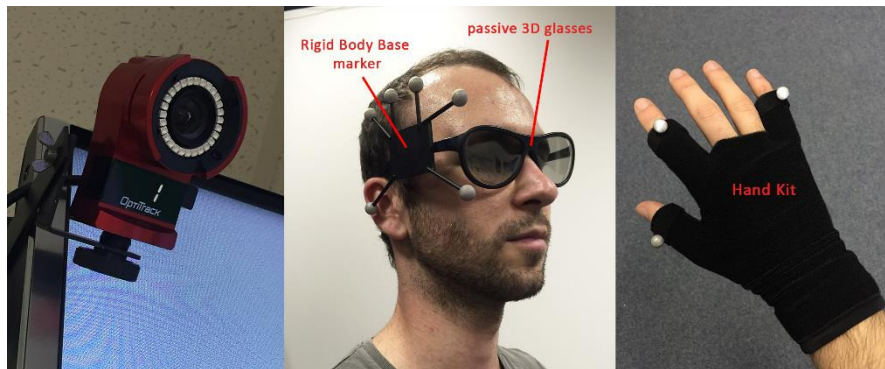
Fig. 4 a) OptiTrack Flex 13 camera system (left), b) rigid body marker for recognition only body movements (middle) c) hand kit marker for finger recognition
