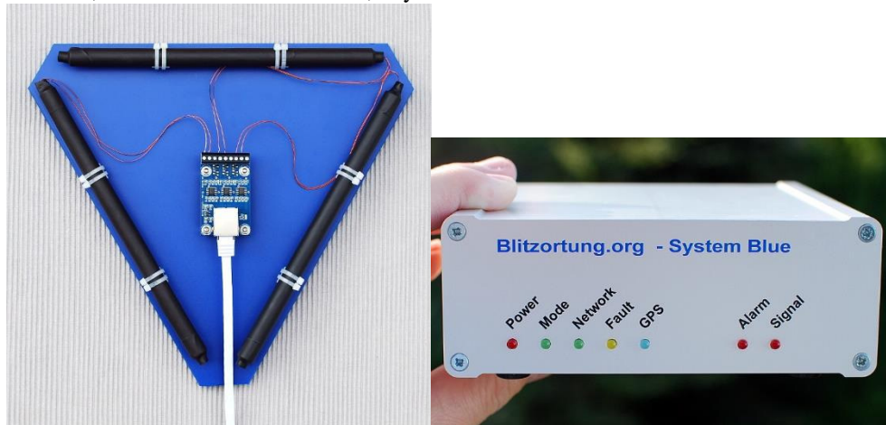
Fig. 1 VLF receiver system of Blitzortung.org [5]
