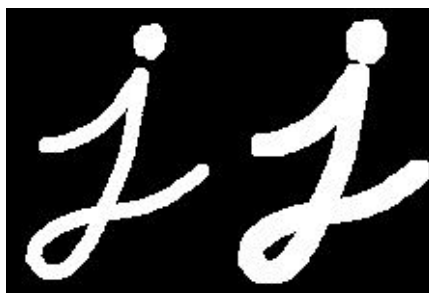
Fig. 3 Morphological operation of dilatation.
