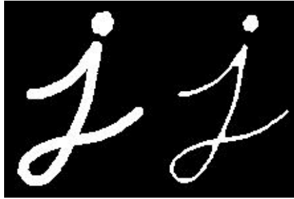
Fig. 1 Morphological operation of erosion.
