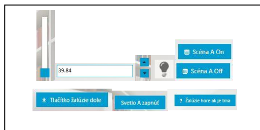
Figure 1. Example of available widgets: dimming, reading, relative dimming, feedback on/off reading, scene, push button, simple write and logical conditional widget
