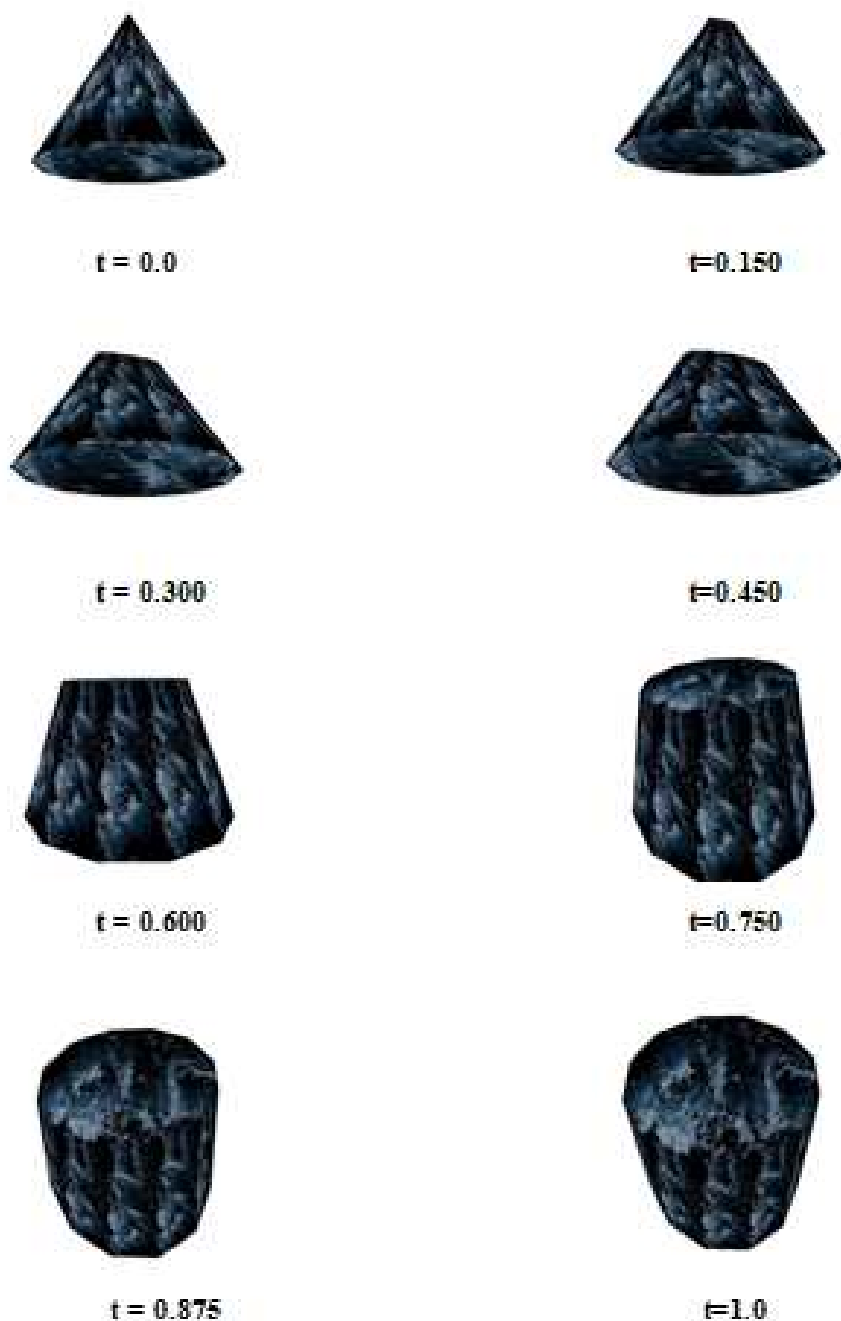
Fig. 3 Example of the morphing by Ferguson's curve - the time course from t = 0 to t = 1
