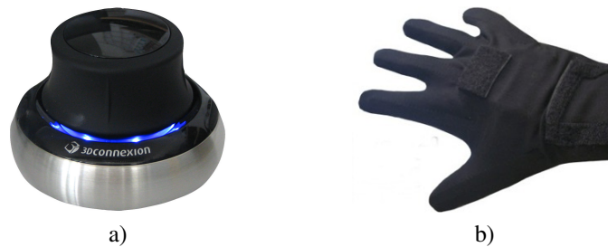
Fig. 3 Supported non-traditional input devices: 3D mouse (a) and data glove (b)
