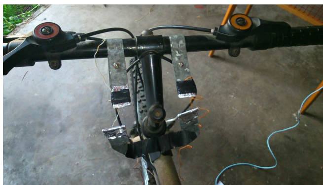
Fig. 2 Sensors on steering wheel
