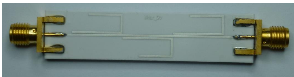
Fig. 2 Fabricated microstrip notch filter (top view)
