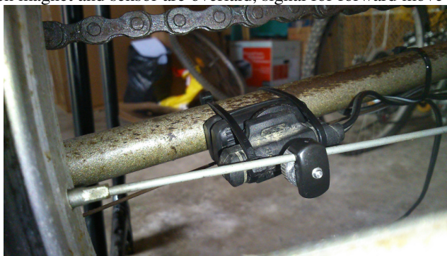
Fig. 3 Sensor on back frame and magnet
