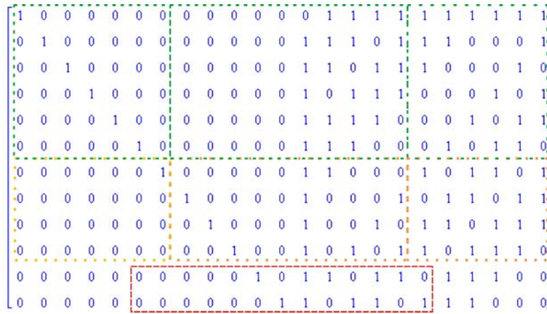
Fig. 3 Binary matrix image representation for obstacle detection system. Note: the red zone is not used in standard image recognition process. This zone is calculated independently and if it is evaluated as an obstacle, the emergency break of the robot is triggered.
